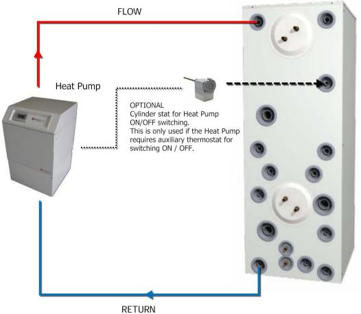
\* Flow and return pipework as per Heat Pump manufacturers recommendation.
