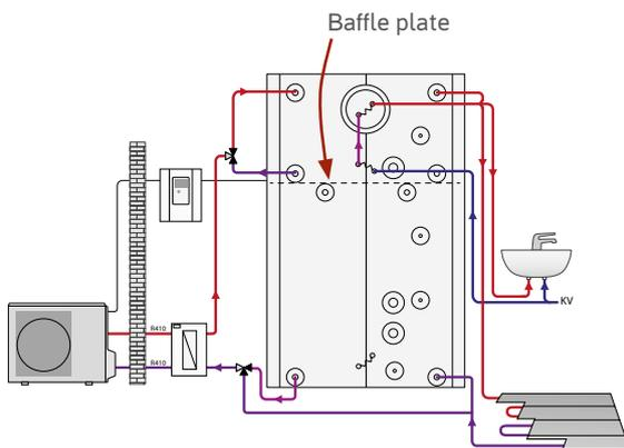
Oval Hybrid 1000 connected to the heat pump, underfloor heating and domestic hot water.
