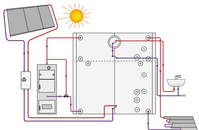
Oval Hybrid 2000 connected to the Jaspi YPV40 wood boiler, Solar panels, underfloor heating and domestic hot water.
