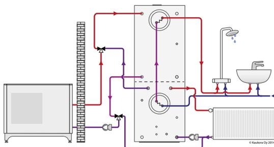
Jaspi Ultrastore 500 connected to a heat pump (Jaspi Comfort Mono), radiators & domestic hot water.
