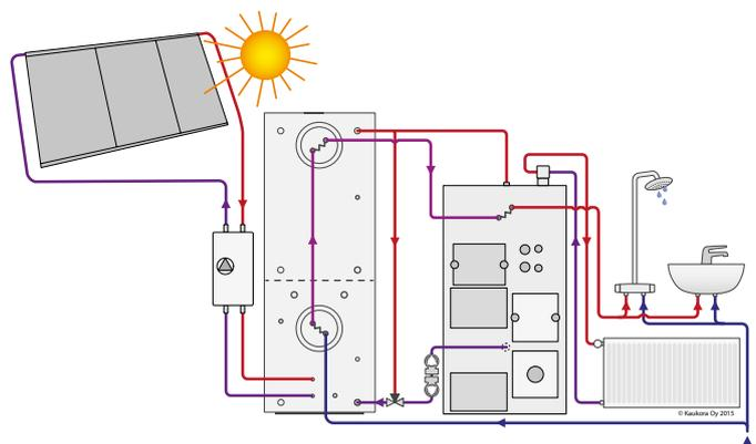
Jaspi Ultrastore 500 connected to a Jaspi Duo multienergy boiler, Solar panels, radiators & domestic hot water.
